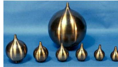
Figure 1. Original Helmholtz resonator set, Different volumes and opening sizes control the resonance frequency.
